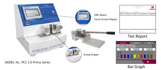
Crease Stiffness Tester is a multi-function stiffness tester, mainly used for measuring cardboard, color box (such as cigarette case cosmetic box) of the indentation force (that is,  $90^{\circ}$  crease of the rebound force), can also measure a variety of cardboard Bending stiffness is achieved on the same instrument with two measurements:  $15^{\circ}$  flexing Degrees and  $90^{\circ}$  crease stiffness. Standards:
